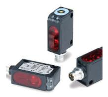
The photoelectric sensor is a device that can determine the presence of an object by measuring how much light reaches its receiver. These sensors often find use in industrial manufacturing facilities. The sensors also help in estimating the distance. The three types of sensors are opposed (through-beam), retro-reflective, and proximity-sensing (diffused).
