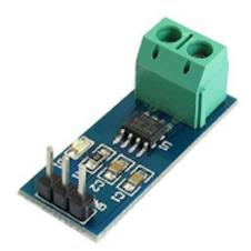
A current sensor is a device to detect the current and convert it into an output voltage. It is easily measurable and proportional to the current through the measured path. Many sensors work for specific current ranges and environmental conditions.
